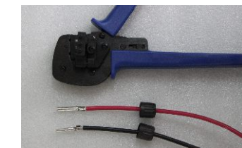
▲ Figure 4.8 Crimp the contact pin to the wire
